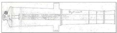
Plan of model 1807 24-pound cast at the Cecil Iron Works, Maryland; weight is marked at 5554 lbs & the trunnion is marked as being 6 inches in diameter. For the plan, the breech ring has been rotated 90 degrees for viewing; it would have been in line with the touch hole. Courtesy, National Archives & Records Administration/Tyrone G. Martin research.
