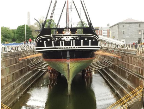
USS Constitution , May 19, 2015, Dry Dock 1 Note: 1995 copper sheathing on hull
